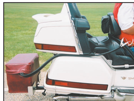
This temporary installation shows how the water lines supply the rider's vest with cool (or warm) water.
