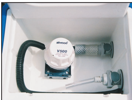
Circulation pump inside the cooler.
